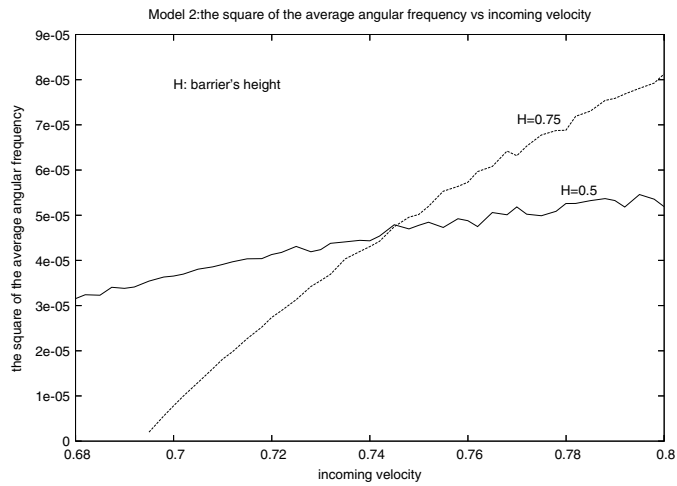
Figure 6. \omega^2 as a function of v_{in} in model 2.
